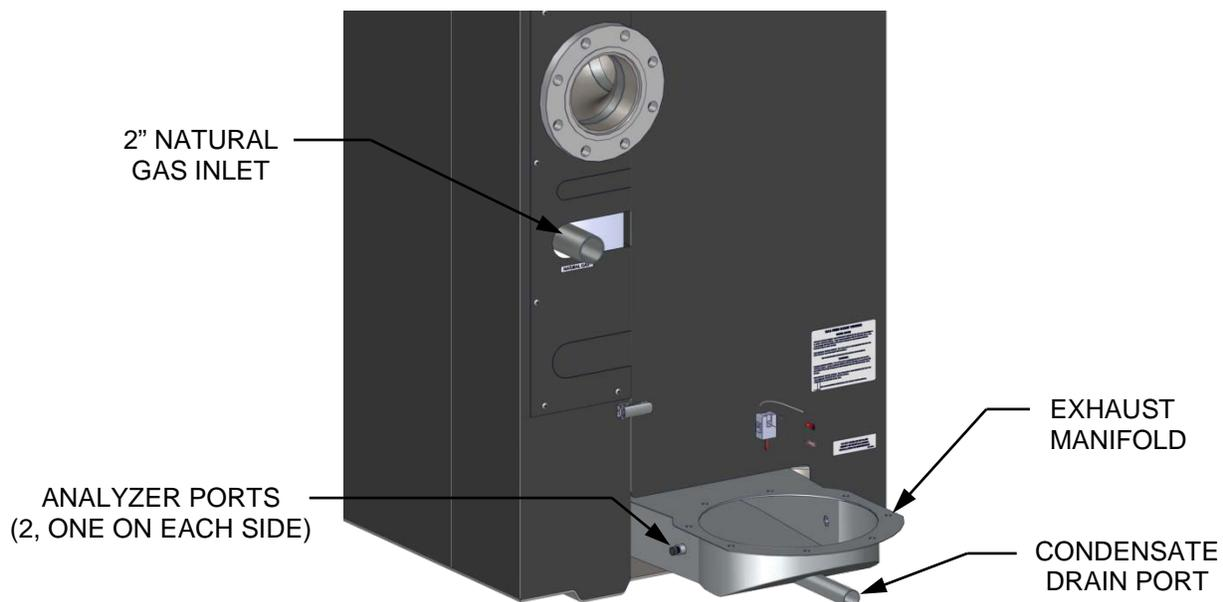
**Figure 2-8: Condensate Drain Connection Location**
