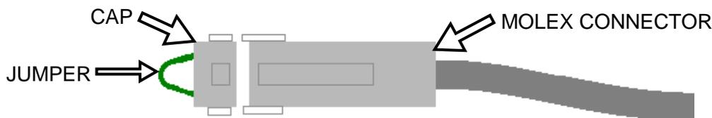
**Figure 2-16: Sequencing Isolation Valve Molex Connector and Jumper Wire**
